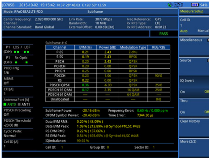
RFoBSAI LTE-FDD signal analyzer window
