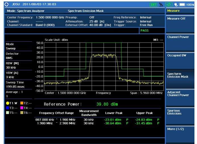
RF analysis — Spectrum Emission Mask
