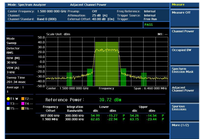
RF analysis — Adjacent Channel Power
