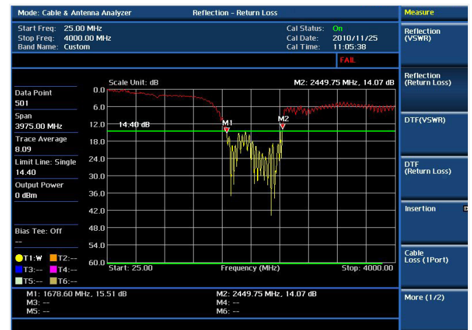
Cable and antenna test — Reflection
