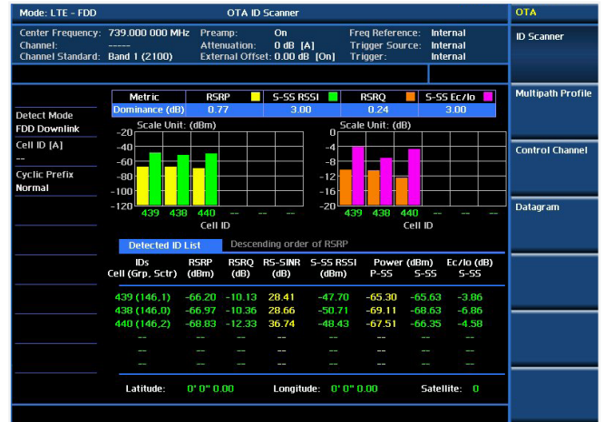
OTA analysis — ID (Channel Scanner)
