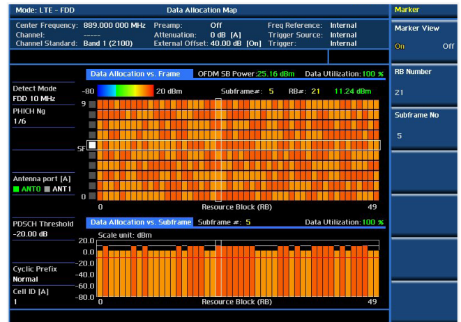
Modulation analysis — Data Allocation Map
