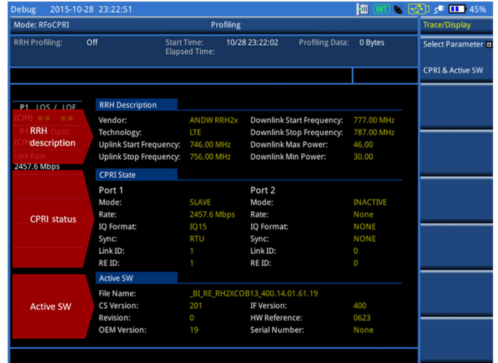
RRH CPRI status and active software
