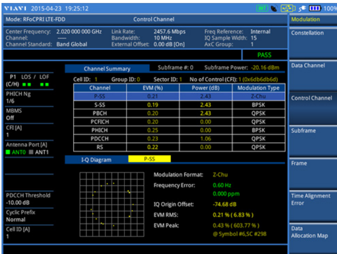
RFoCPRI — DL signal analysis window
